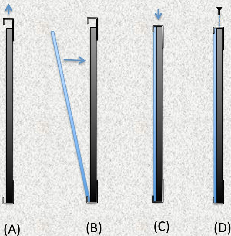
Step 9: Slide the provided insert into the top of your now fully assembled unit.
