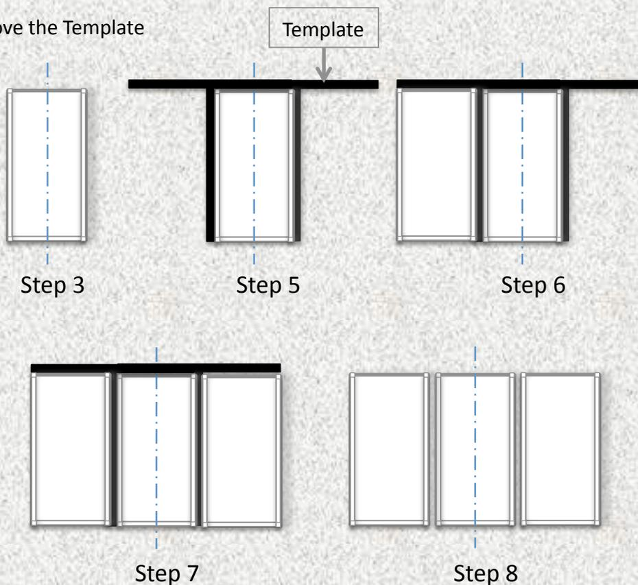
Step 8: The clips on the bottom are ready as is. Push the top clips up (A). Seat the glass into the bottom clips centering the glass side to side. Tilt the glass into position (B). Slide the top clips down (C) capturing the top edge of the glass. Use supplied ½" painted screw to secure the top clips (D).
